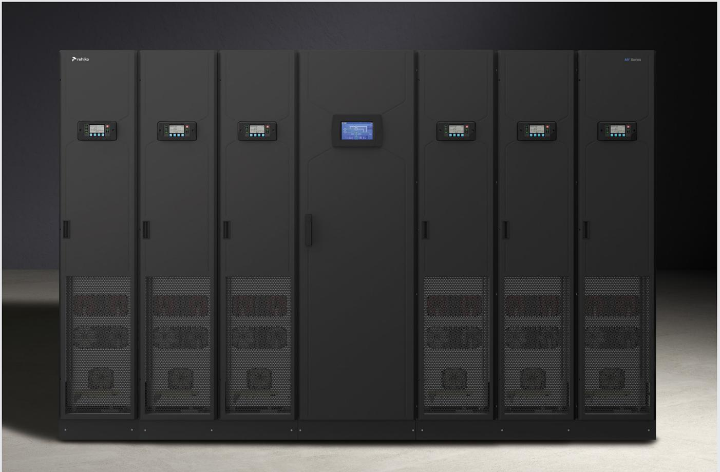
A 1.5MW Rehlko MF Series with a central connections cabinet flanked by six 250kW modules, each containing all elements of a UPS.
